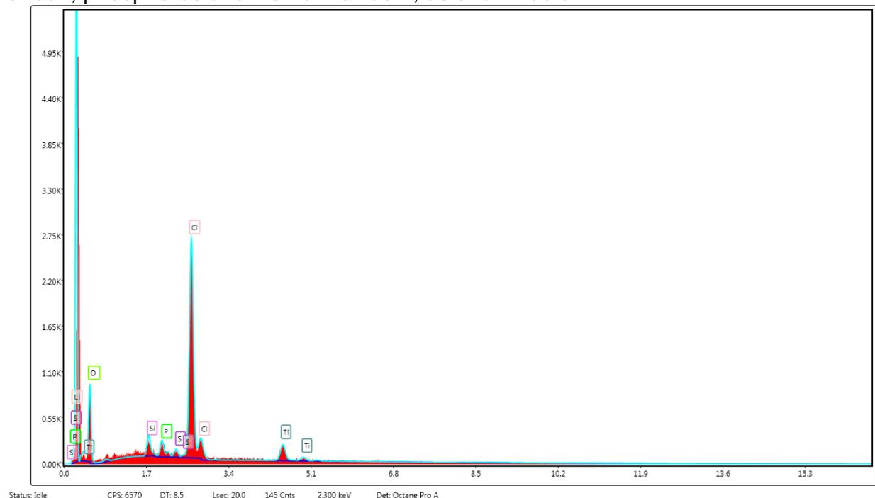
The basecoat for ITEM 4 (spectrum shown below), however, could be differentiated from the basecoat of ITEM 1 on the basis of phosphorus, which appeared to be absent in ITEM 4, and the relative abundance of chlorine.
