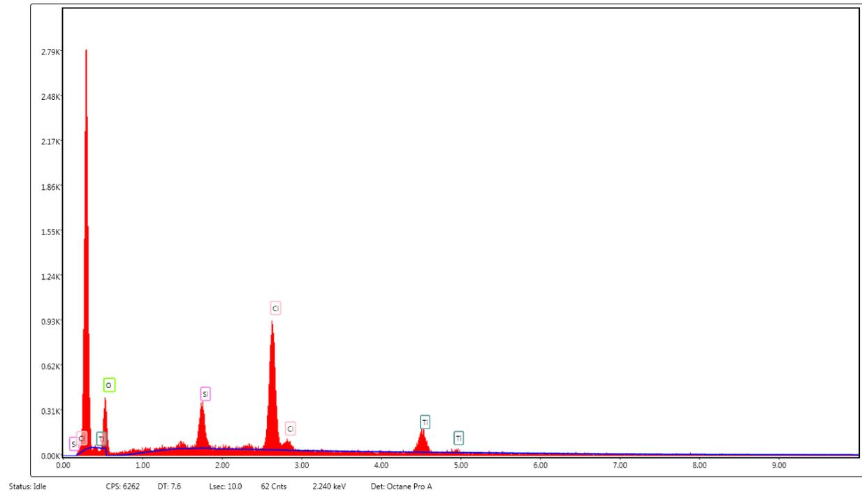
Surfacer layers for ITEMS 1, 2, 3 and 4 could not be differentiated nor could the primer layers. Exemplar spectra are provided below.
