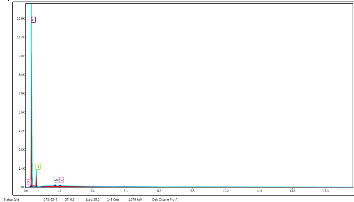
The basecoat for ITEMS 1, 2 and 3 showed an abundance of chlorine with traces of silicon, phosphorus and titanium evident, as shown below.
